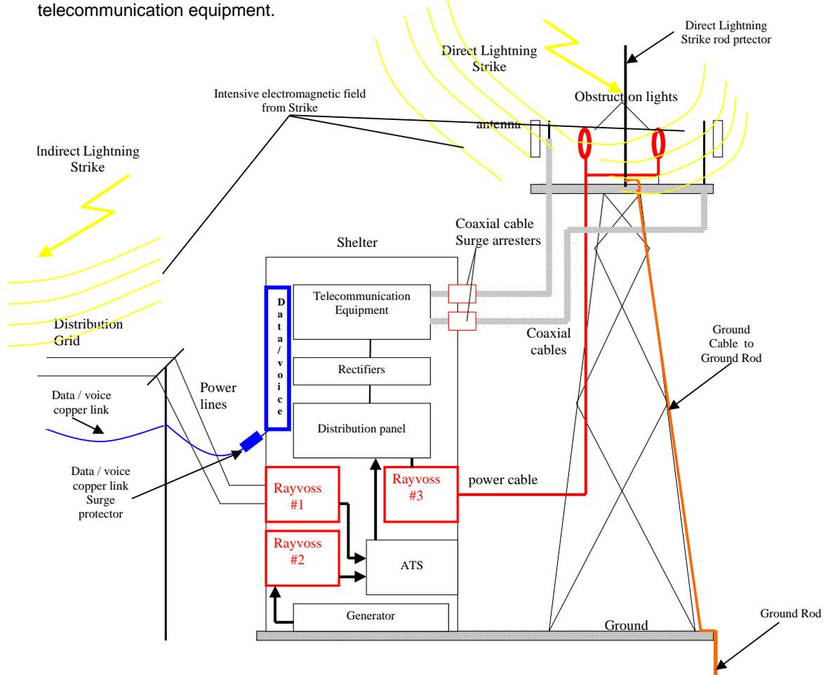
The equipment is subjected to surges caused by **direct lightning strikes** on the tower structure, as well as **indirect strikes** which induce surges on the power lines, data/voice lines and also Tx/Rx coaxial lines. The protection from the effect of these two types of lightning strikes is explained below:
